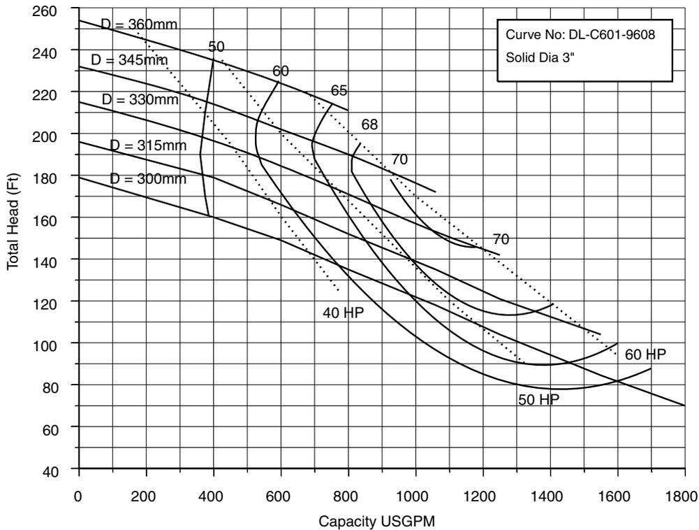
**200x150DDL611 (15HP) Synchronous Speed: 1800 RPM 8 inch Suction 6 inch Discharge**
