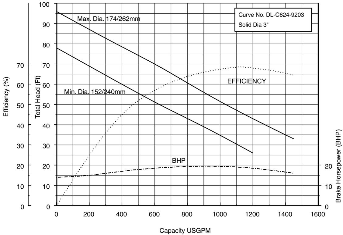
**200x150DDL618 (25HP) Synchronous Speed: 1800 RPM 8 inch Suction 6 inch Discharge**
