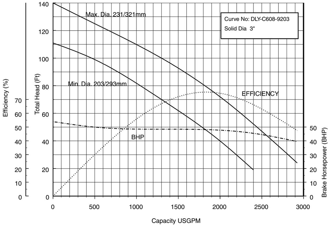
**250x250DDL645 (60HP) Synchronous Speed: 1800 RPM 10 inch Suction 10 inch Discharge**
