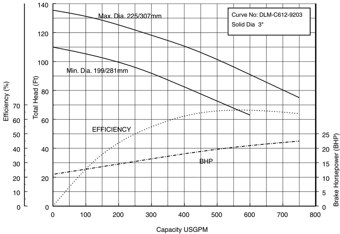
**100x80DDL622 (30HP) Synchronous Speed: 1800 RPM 4 inch Suction 3 inch Discharge**
