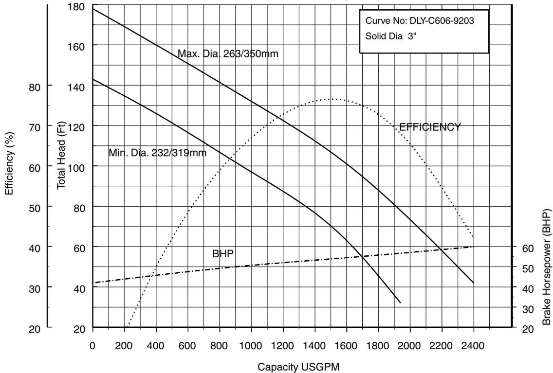
**250x250DDL630 (40HP) Synchronous Speed: 1800 RPM 10 inch Suction 10 inch Discharge**
