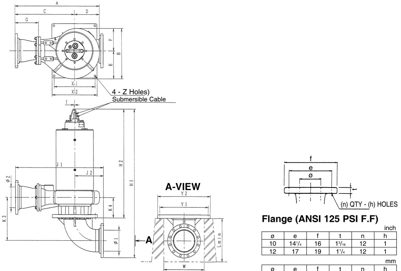
*Note: Discharge can be rotated in 30 increments.*
