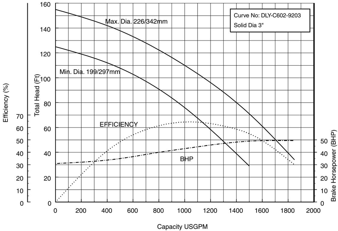
**200x150DDL645 (60HP) Synchronous Speed: 1800 RPM 8 inch Suction 6 inch Discharge**
