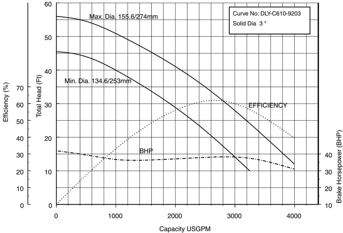
**300x300DDL637 (50HP) Synchronous Speed: 1800 RPM 12 inch Suction 12 inch Discharge**
