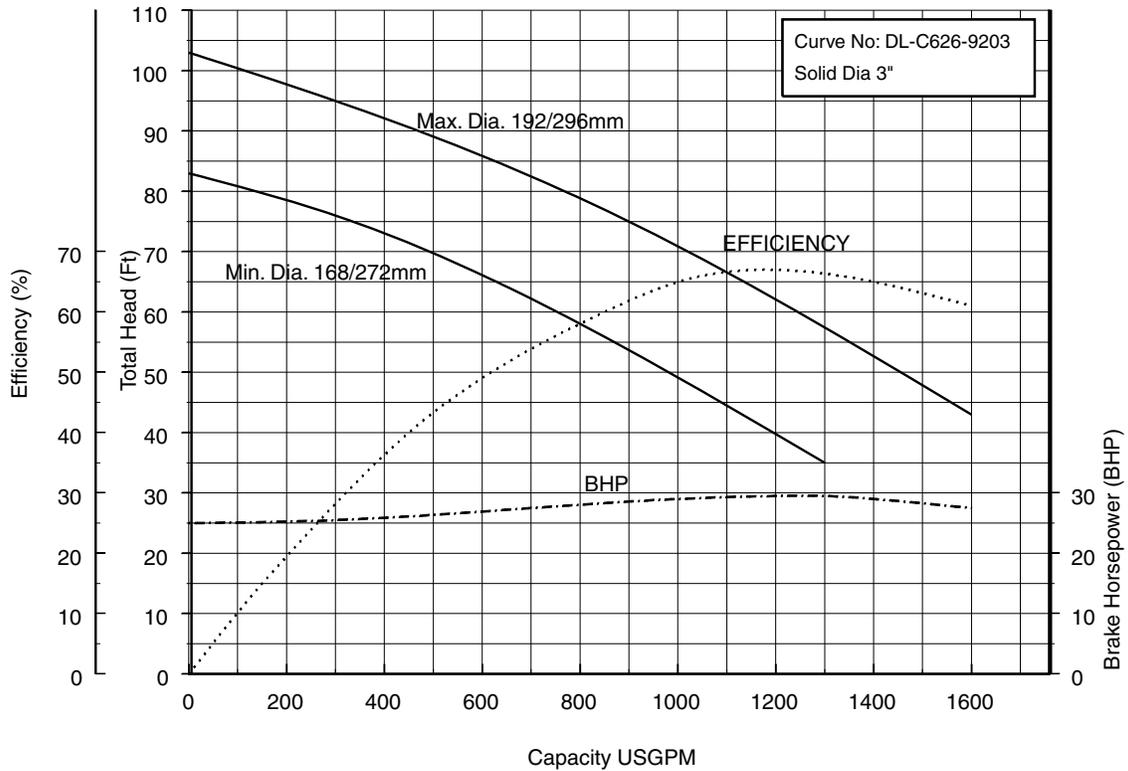
**200x150DDL630 (40HP) Synchronous Speed: 1800 RPM 8 inch Suction 6 inch Discharge**
