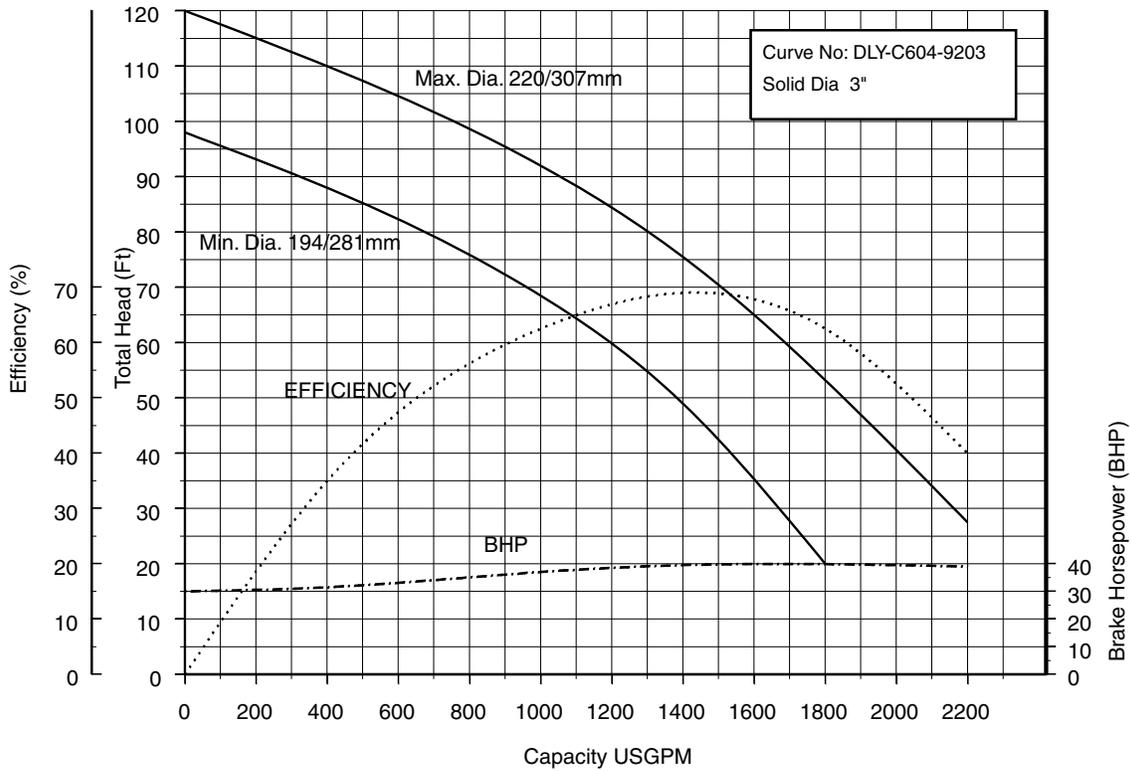
**200x200DDL637 (50HP) Synchronous Speed: 1800 RPM 8 inch Suction 8 inch Discharge**
