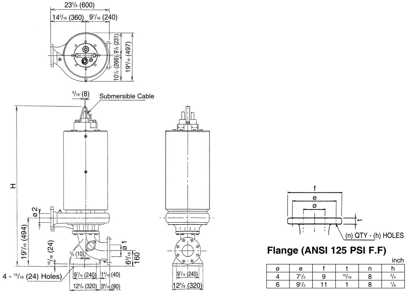
*Note: Discharge can be rotated in 45 increments.*
