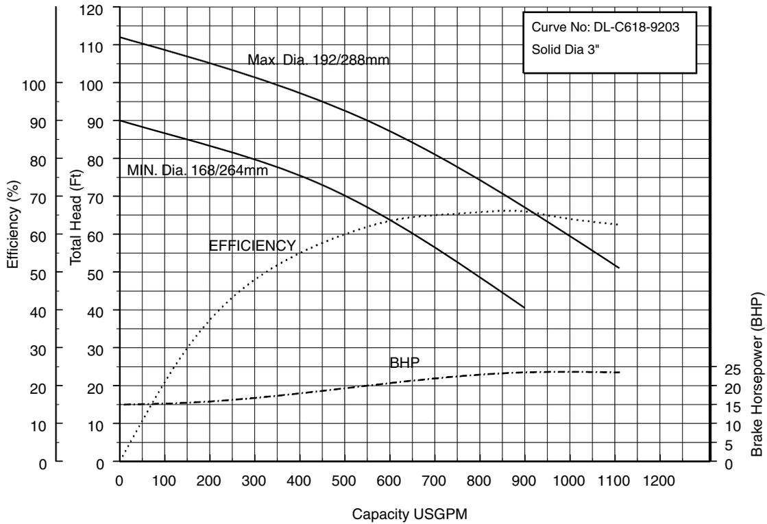
**150x100DDL622 (30HP) Synchronous Speed: 1800 RPM 6 inch Suction 4 inch Discharge**
