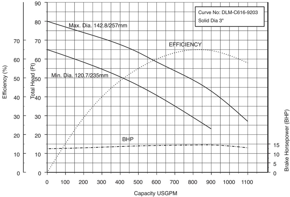
**150x100DDL615 (20HP) Synchronous Speed: 1800 RPM 6 inch Suction 4 inch Discharge**
