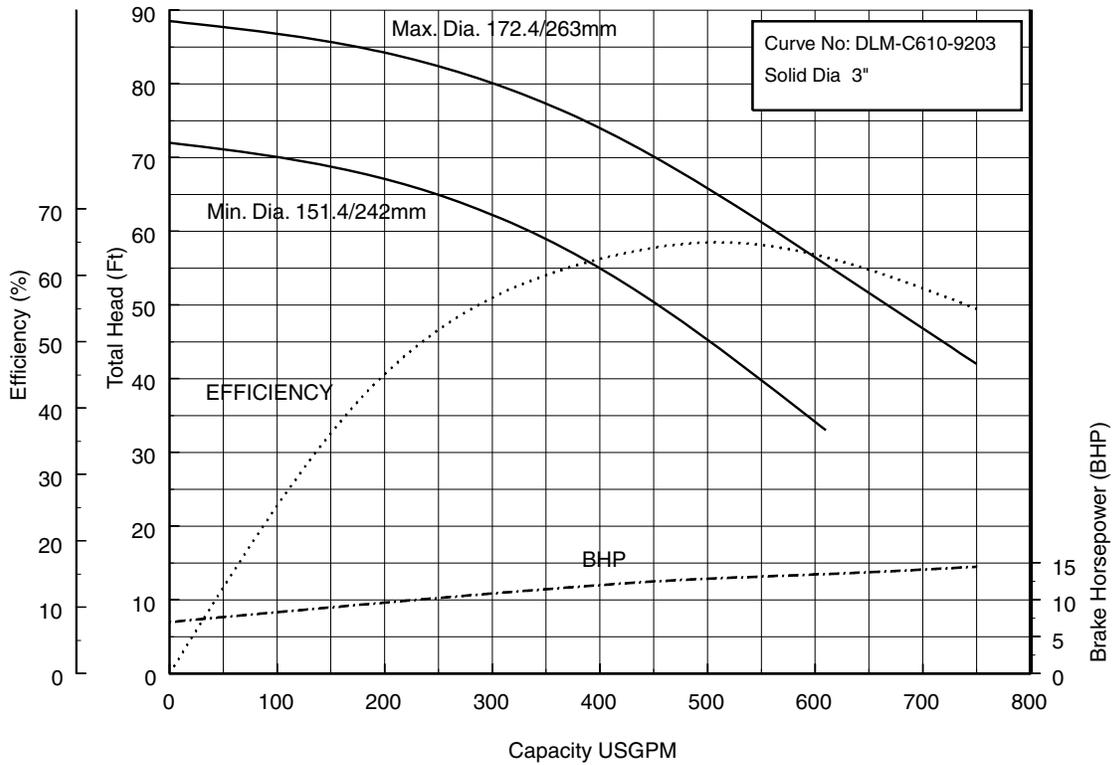
**100x80DDL615 (20HP) Synchronous Speed: 1800 RPM 4 inch suction 3 inch Discharge**
