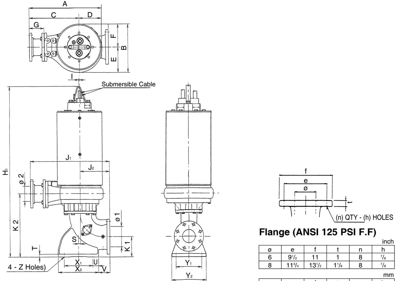
Note: Discharge can be rotated in 30 increments.
