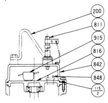
Motors purchased as a complete unit. Parts No. 915 is not installed for Model DSHU. Parts No. 117-4 is not installed, No. 115-2 is installed 2 pcs. for  $7^{1/2}$ -10HP.
