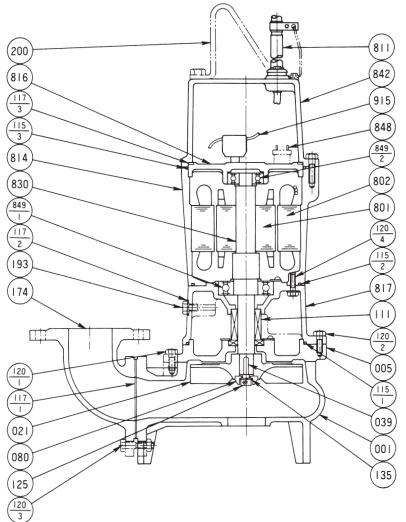
Motors are purchased as a complete unit. Parts No. 915 is not installed for DVSHU.
