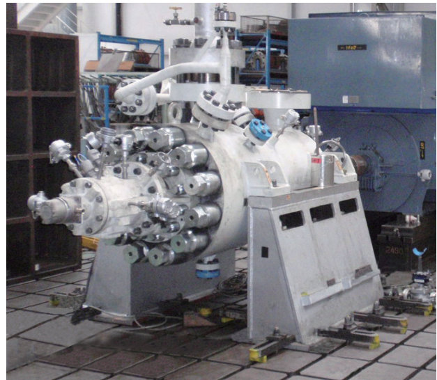
Fig. 4 External appearance of CO 2 injection pump
