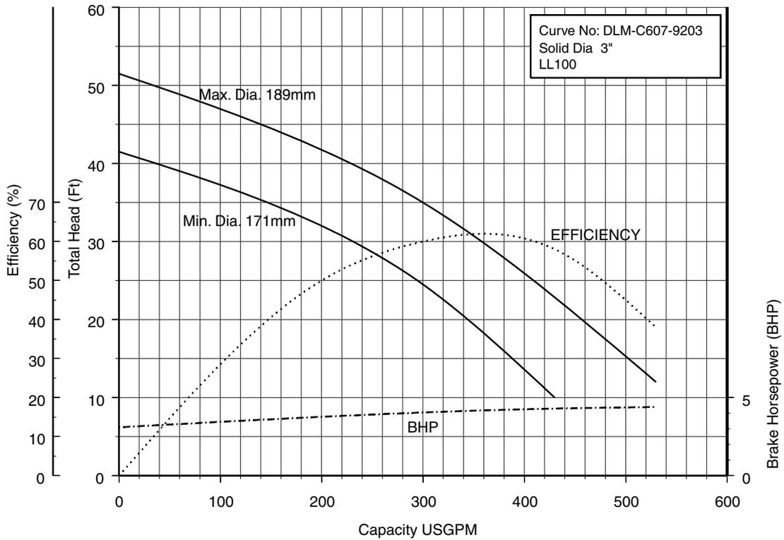
**100DLF65.5 (7½HP) Synchronous Speed: 1800 RPM**
