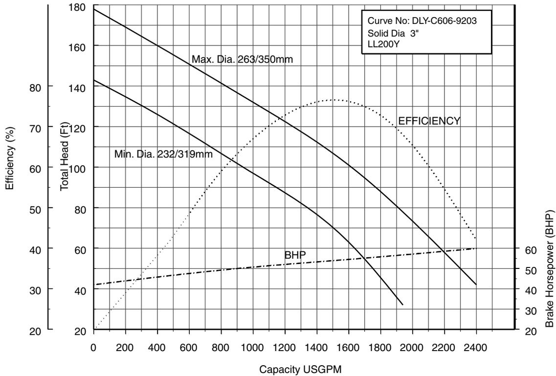
**250DLF611 (15HP) Synchronous Speed: 1800 RPM**
