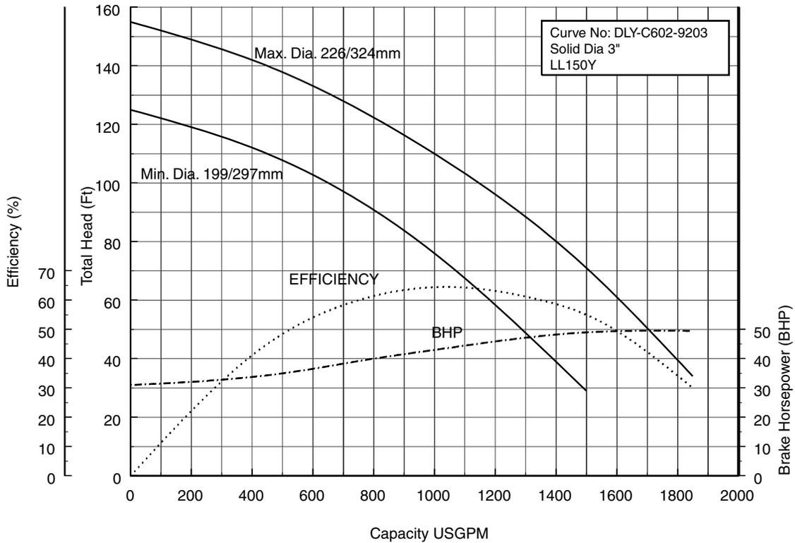
**150DLF645 (60HP) Synchronous Speed: 1800 RPM**
