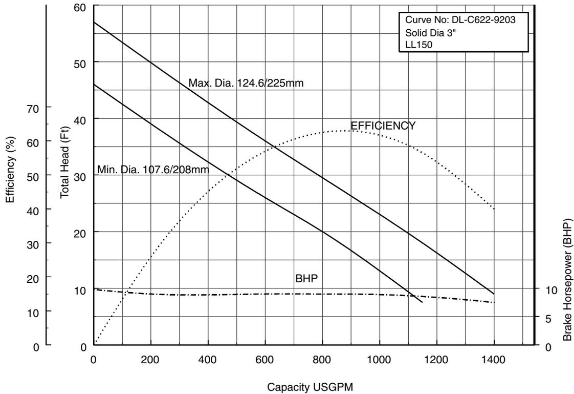
**150DLF611 200DLF611 (15HP) Synchronous Speed: 1800 RPM**
