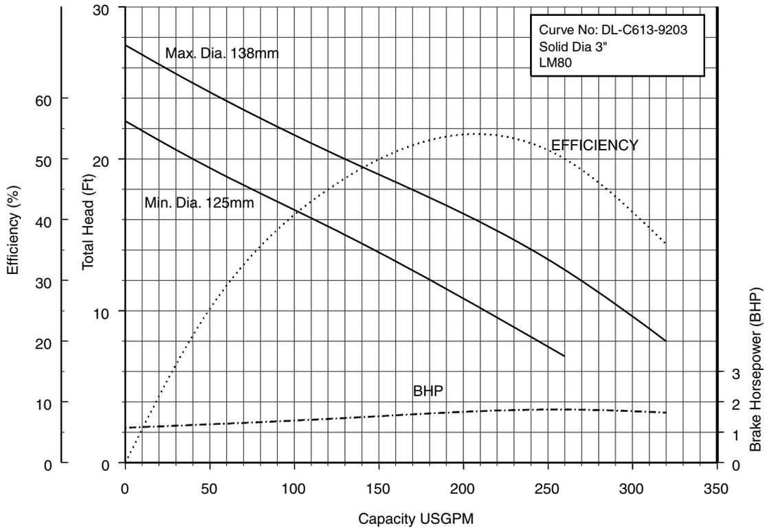
**100DLF62.2 (3HP) Synchronous Speed: 1800 RPM**
