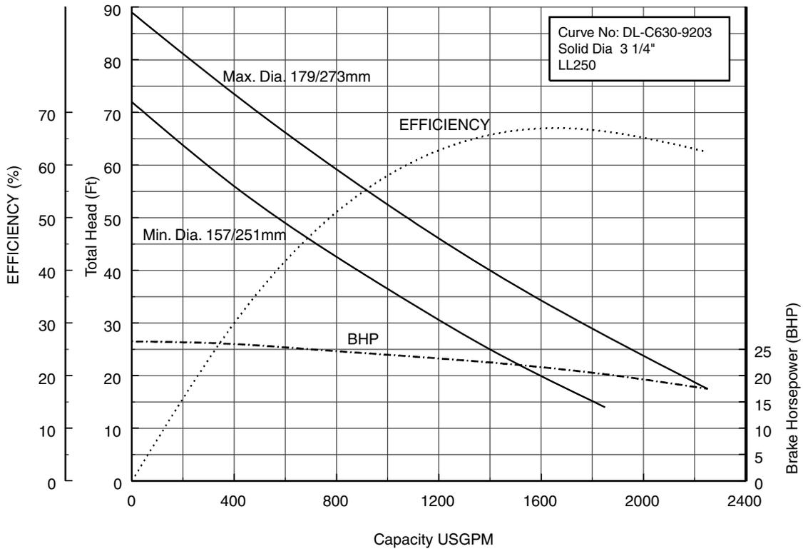
**250DLF622 (30HP) Synchronous Speed: 1800 RPM**
