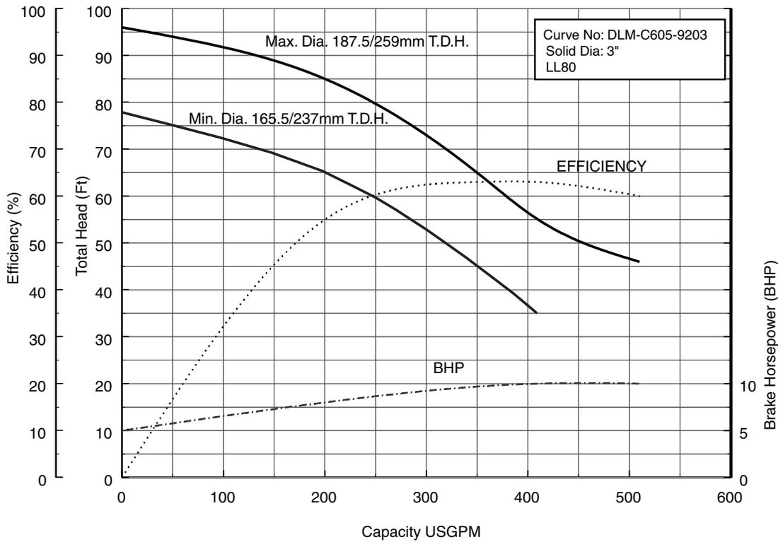
**80DLF611 (15HP) Synchronous Speed: 1800 RPM**
