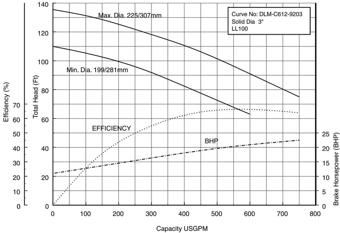
80DLF622 (30HP) Synchronous Speed: 1800 RPM
