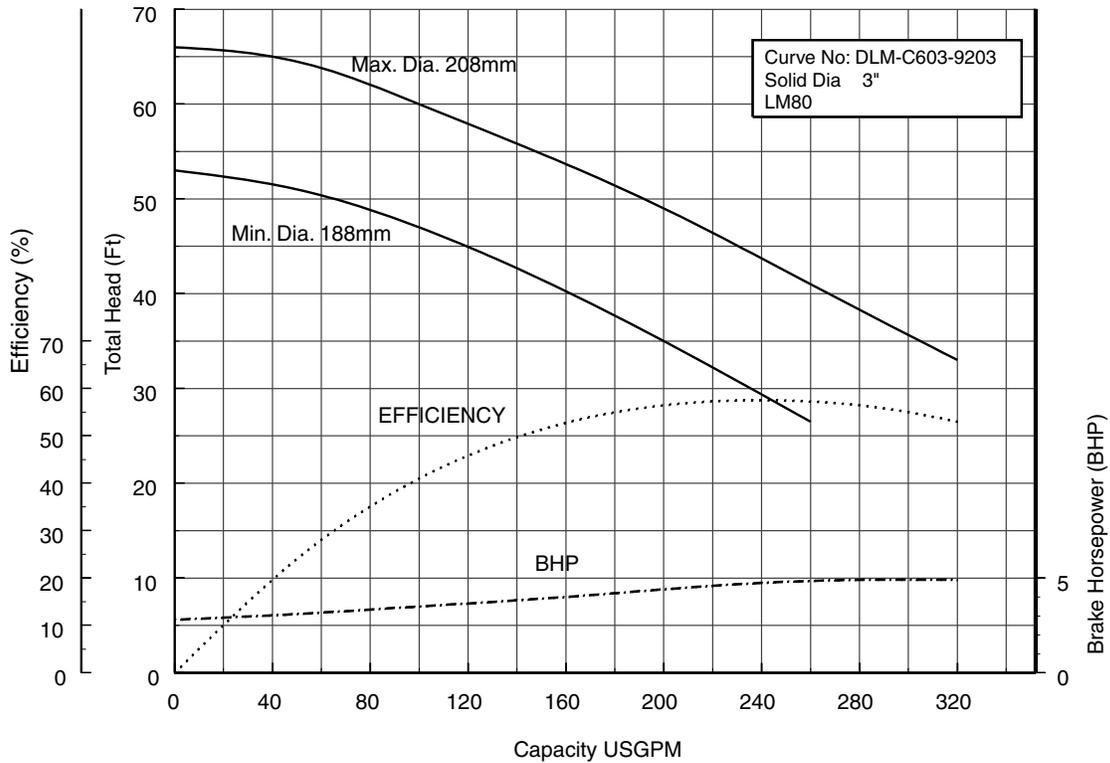
**80DLF65.5 (7½HP) Synchronous Speed: 1800 RPM**
