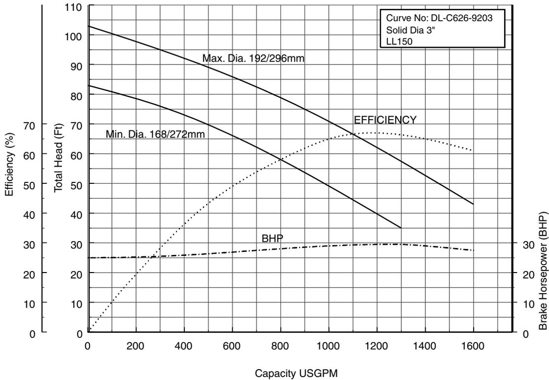
**150DLF630 (40HP) Synchronous Speed: 1800 RPM**
