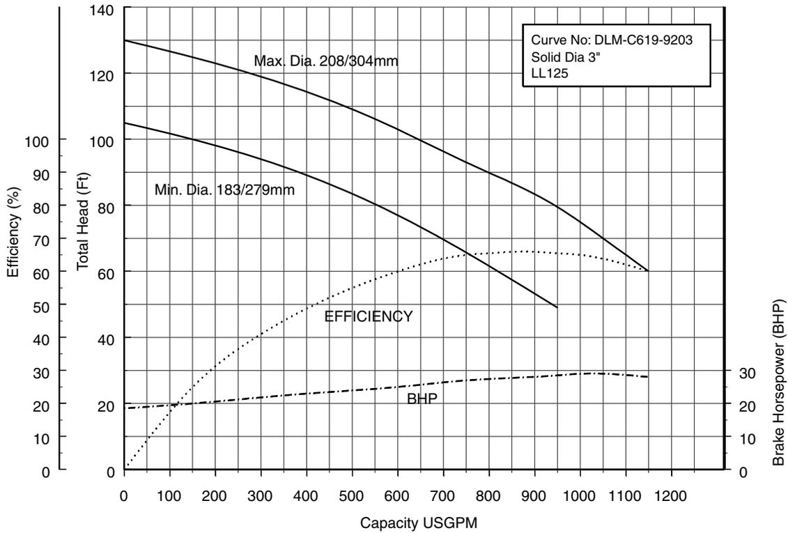
**100DLF630 to 645 (40-60HP) Synchronous Speed: 1800 RPM**
