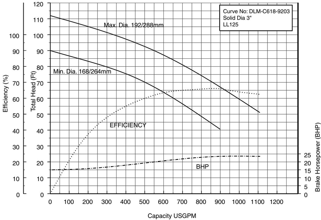
100DLMF622 (30HP) Synchronous Speed: 1800 RPM
