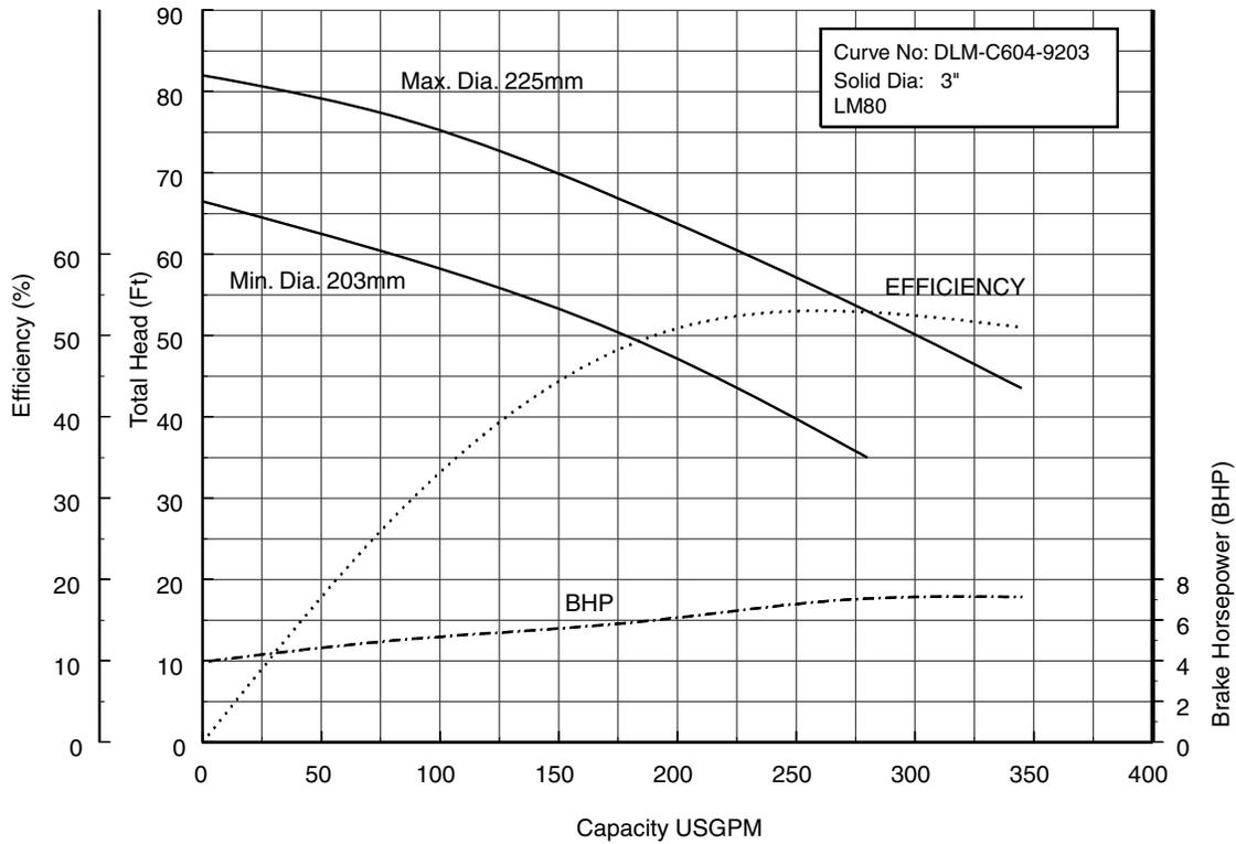
**80DLF67.5 (10HP) Synchronous Speed: 1800 RPM**
