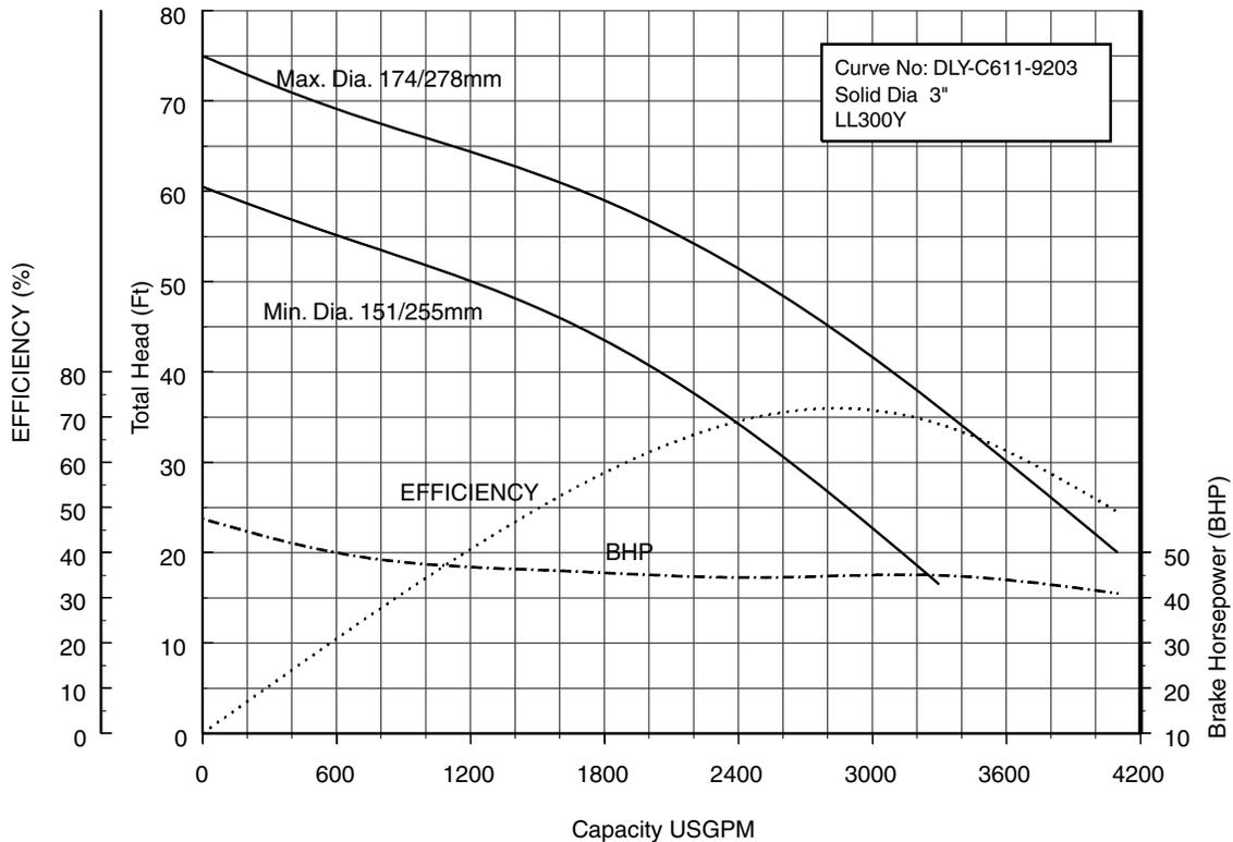
**300DLF645 (60HP) Synchronous Speed: 1800 RPM**
