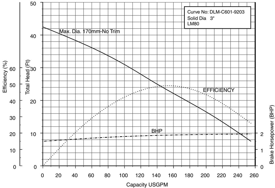
**80DLF62.2 (3HP) Synchronous Speed: 1800 RPM**
