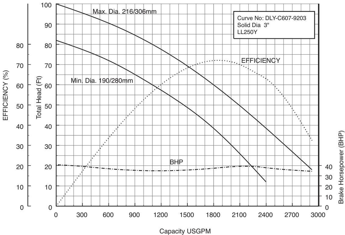
**250DLF637 (50HP) Synchronous Speed: 1800 RPM**
