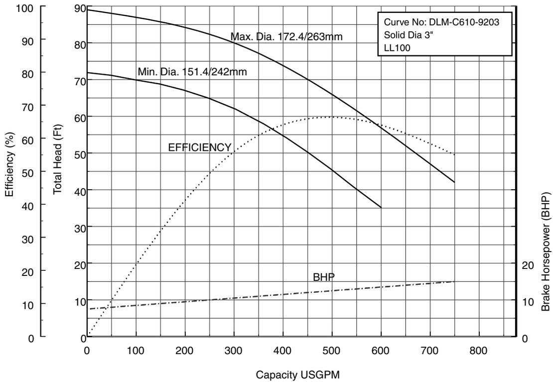
100DLF615 (20HP) Synchronous Speed: 1800 RPM
