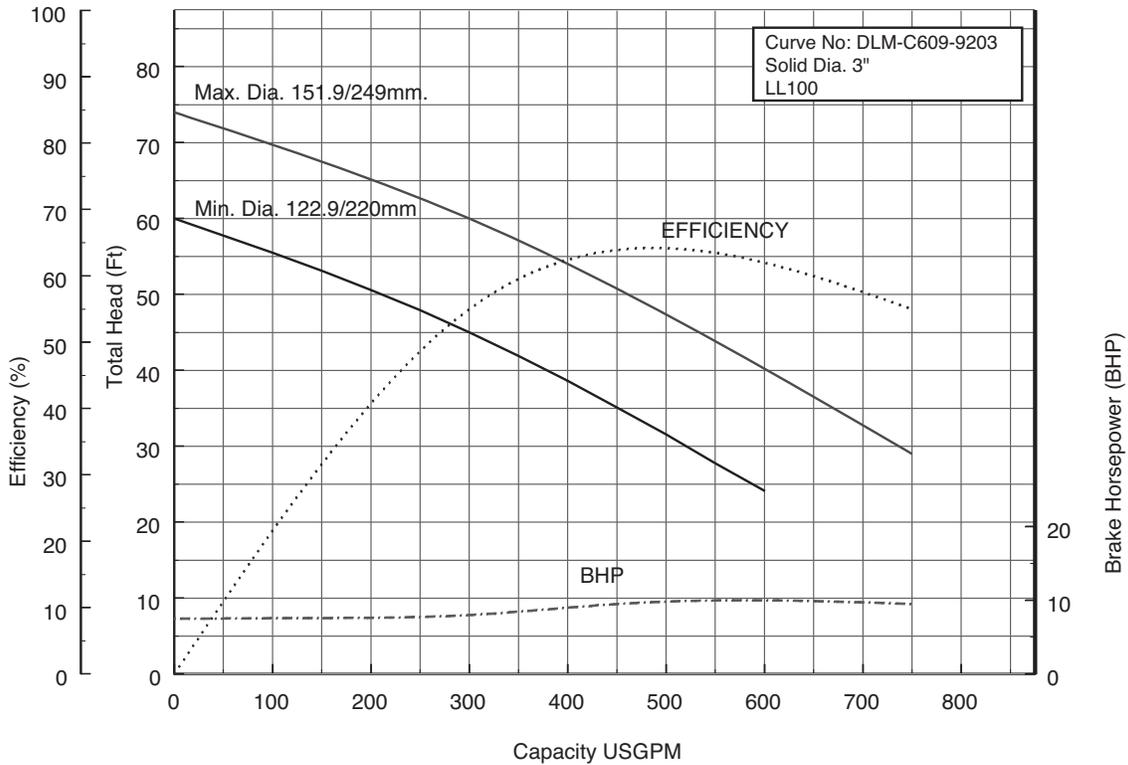
**100DLF611 (15HP) Synchronous Speed: 1800 RPM**
