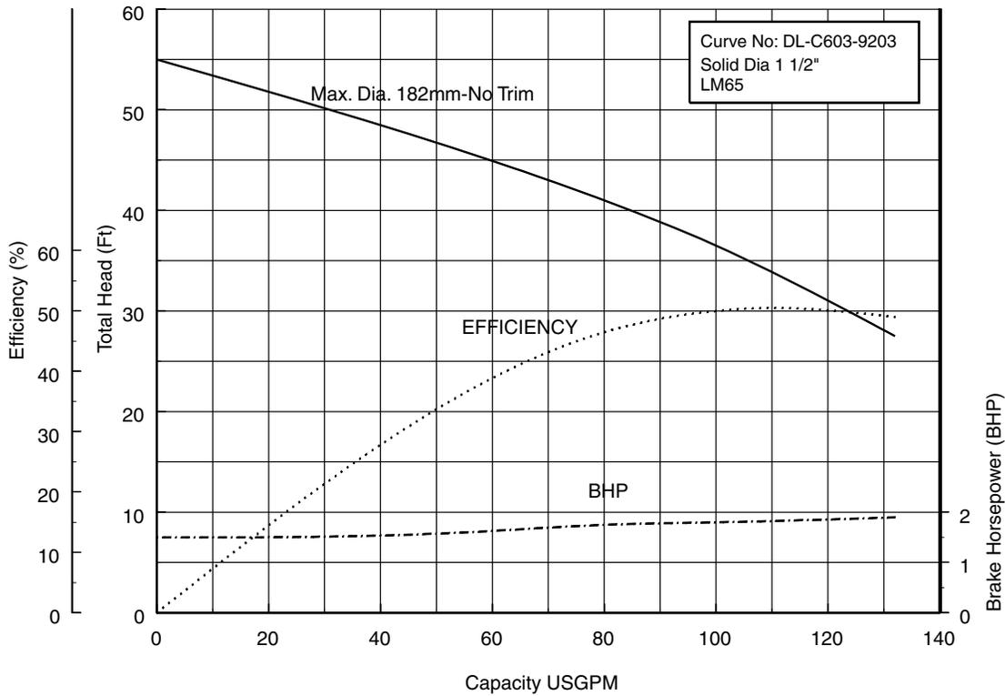
**80DLF61.5 (2HP) Synchronous Speed: 1800 RPM**
