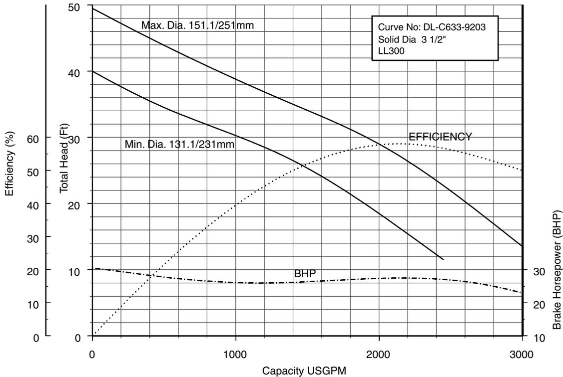
**300DLF630 (40HP) Synchronous Speed: 1800 RPM**
