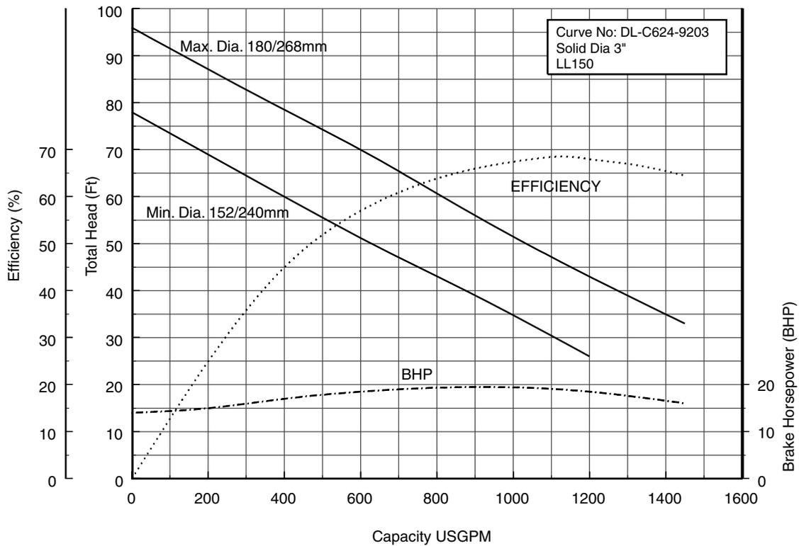
**150DLF618 200DLF618 (25HP) Synchronous Speed: 1800 RPM**
