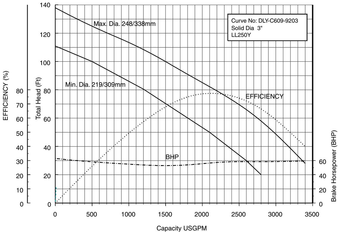
**300DLF618 (25HP) Synchronous Speed: 1800 RPM**
