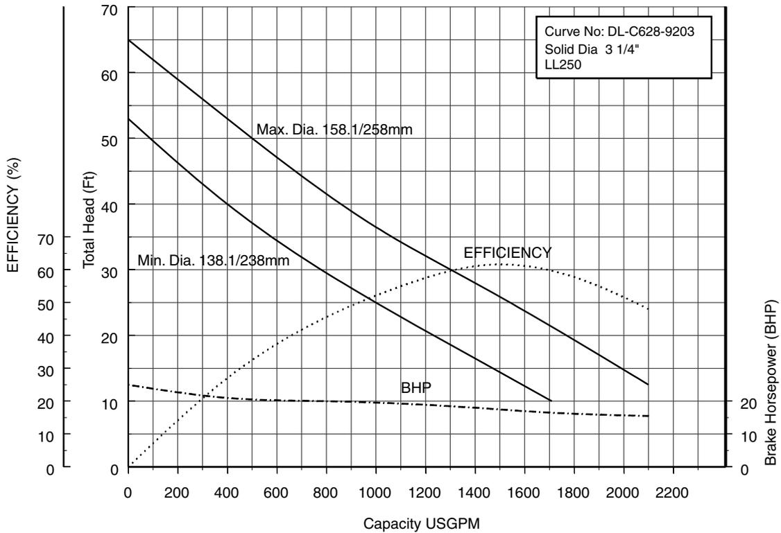
250DLCF615 (20HP) Synchronous Speed: 1800 RPM
