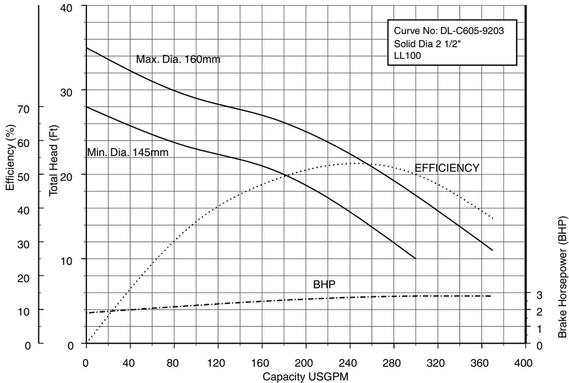
100DLF63.7 (5HP) Synchronous Speed: 1800 RPM
