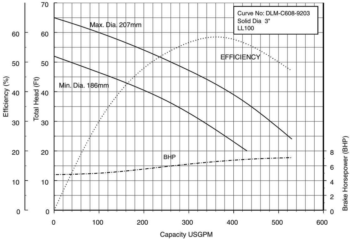
100DLF67.5 (10HP) Synchronous Speed: 1800 RPM
