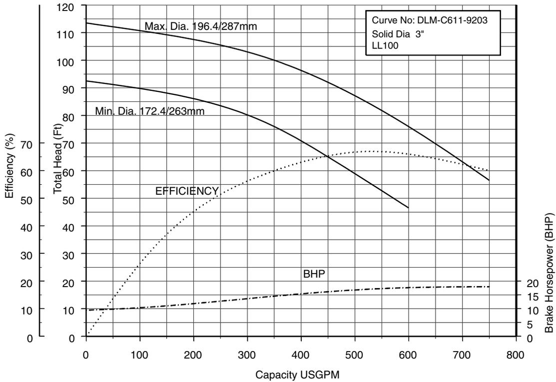
**100DLMF618 (25HP) Synchronous Speed: 1800 RPM**
