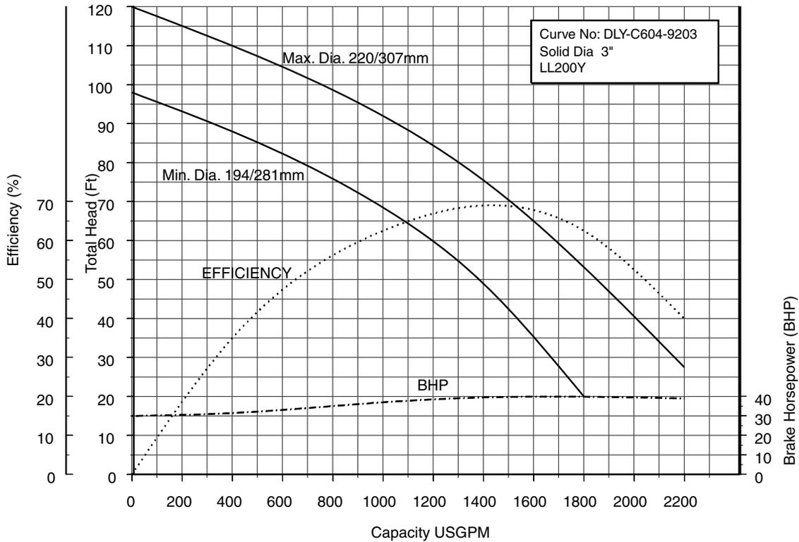
**200DLF637 (50HP) Synchronous Speed: 1800 RPM**
