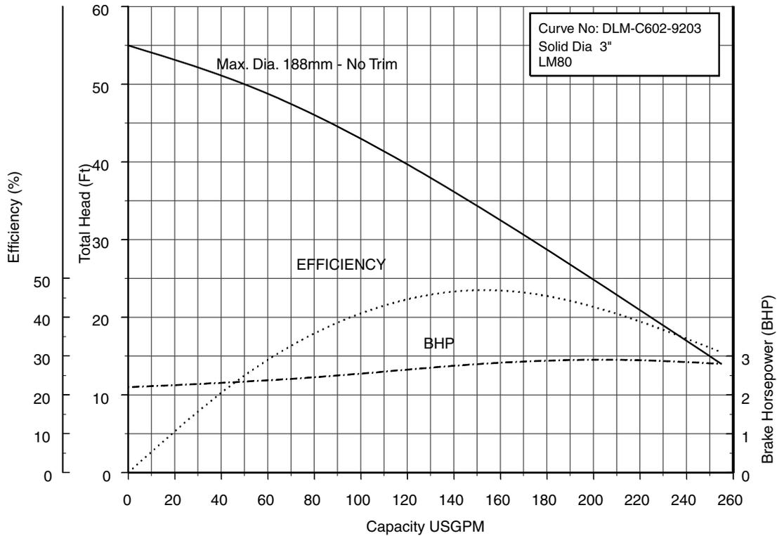
**80DLF63.7 (5HP) Synchronous Speed: 1800 RPM**
