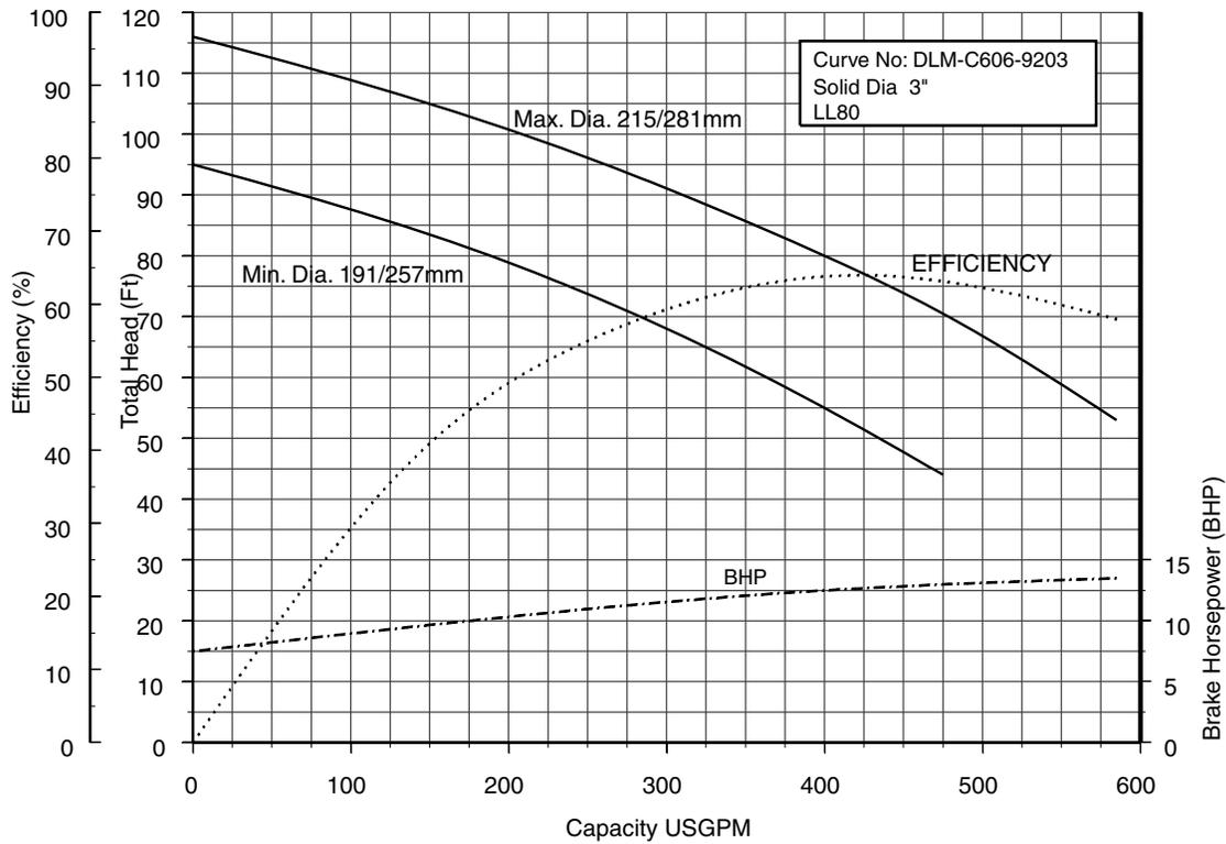
**80DLF615 (20HP) Synchronous Speed: 1800 RPM**
