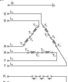
$$\begin{split} G &= GRN \\ L_1 &= RED - T_1 \\ L_2 &= WHT - T_2 \\ L_3 &= BLK - T_3 \\ L_5 &= WHT - T_{10} \\ L_6 &= BLK - T_{11} \\ L_4 &= RED - T_{12} \\ T_4 &= T_7 \\ T_5 &= T_8 \\ T_6 &= T_9 \\ P_1 &= RED \\ P_2 &= WHT \\ P_3 &= BLK \\ P_4 &= OR \\ G &= GRN \\ \end{split}$$
