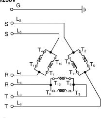
$$\begin{split} & L_1 - \text{RED} - T_1 - T_7 \\ & L_2 - \text{WHT} - T_2 - T_8 \\ & L_3 - \text{BLK} - T_3 - T_9 \\ & L_5 - \text{WHT} - T_4 - T_{10} \\ & L_6 - \text{BLK} - T_5 - T_{11} \\ & L_4 - \text{RED} - T_6 - T_{12} \\ & P_1 - \text{RED} \\ & P_2 - \text{WHT} \\ & P_3 - \text{BLK} \\ & P_4 - \text{ORG} \\ & G - \text{GRN} \end{split}$$
