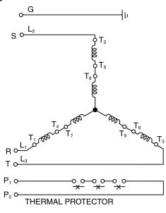
$$\begin{aligned} &G-GRN\\ &L_1-RED-T_1\\ &L_2-WHT-T_2\\ &L_3-BLK-T_3\\ &T_4-T_7\\ &T_5-T_8\\ &T_6-T_9\\ &P_1-RED\\ &P_2-WHT\\ &P_3-BLK\\ &P_4-ORG\\ &G-GRN \end{aligned}$$
