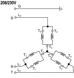
$$\begin{aligned} & G - GRN \\ & L_1 - RED - T_1 - T_7 \\ & L_2 - WHT - T_2 - T_8 \\ & L_3 - BLK - T_3 - T_9 \\ & T_4 - T_5 - T_6 \end{aligned}$$
