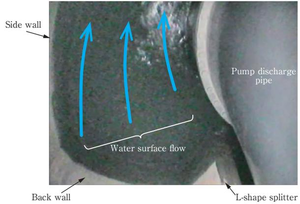
**Fig. 14** Water surface flow adjacent to pump suction pipe
