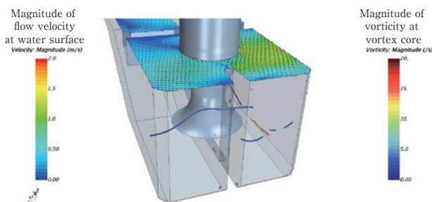
Fig. 17 CFD analysis results of pump sump
