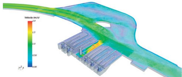
**Fig. 15** CFD analysis results of pump sump along with balancing reservoir
