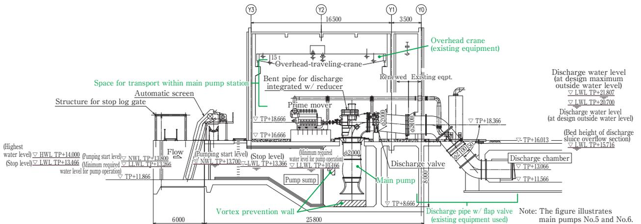
Fig. 3 Cross section of pump station (after renewal)
