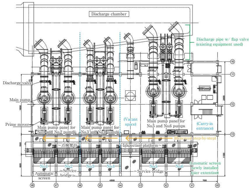
Fig. 2 (b) Plan view of pump station layout (after renewal)
