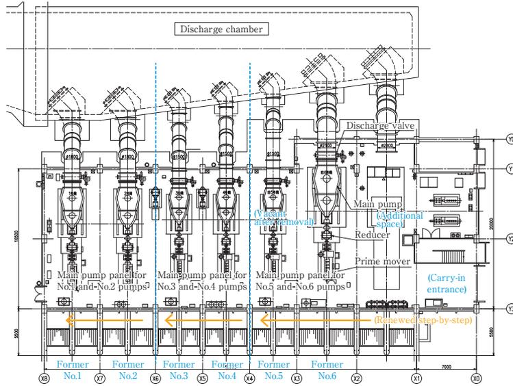
Fig. 2 (a) Plan view of pump station layout (before renewal)
