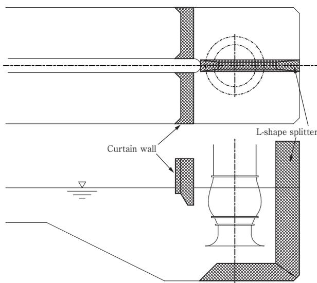
**Fig. 11** Configuration of vortex suppression devices
