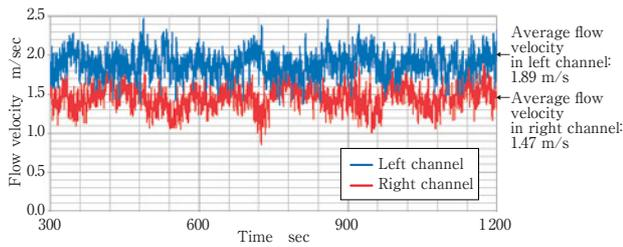
**Fig. 13** Flow velocity in No.4 pump sump
