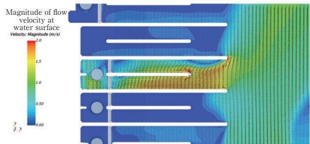
**Fig. 16** Inflow into No.4 pump sump
